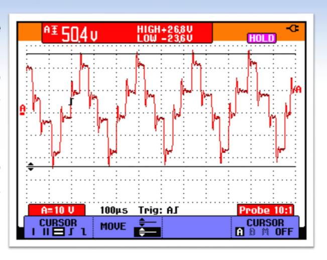
**Important note:** This six-step or square wave is what is seen when there is no bearing discharge and the peak to peak shaft voltage is at it's maximum level. The continued voltage will eventually overcome the dielectric in most bearings and begin discharging.
