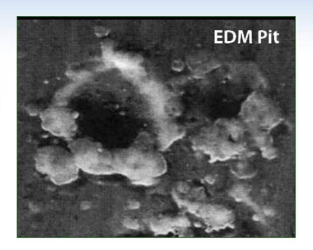
When this event happens, temperatures are hot enough to melt bearing steel and severely damage the bearing lubrication.
