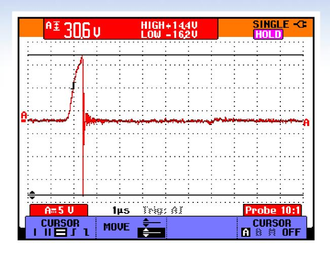
These voltages, which can register 10-40 volts peak, are easily measured by touching an oscilloscope probe to the shaft while the motor is running.
