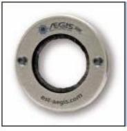
Mounting with holes and countersunk screws Shaft diameter: 8 mm to 153 mm M3 x 14 countersunk screws 2 holes for shaft diameters up to 99 mm 3 holes for larger diameter
