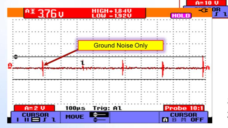
Shaft Voltage Reading:
