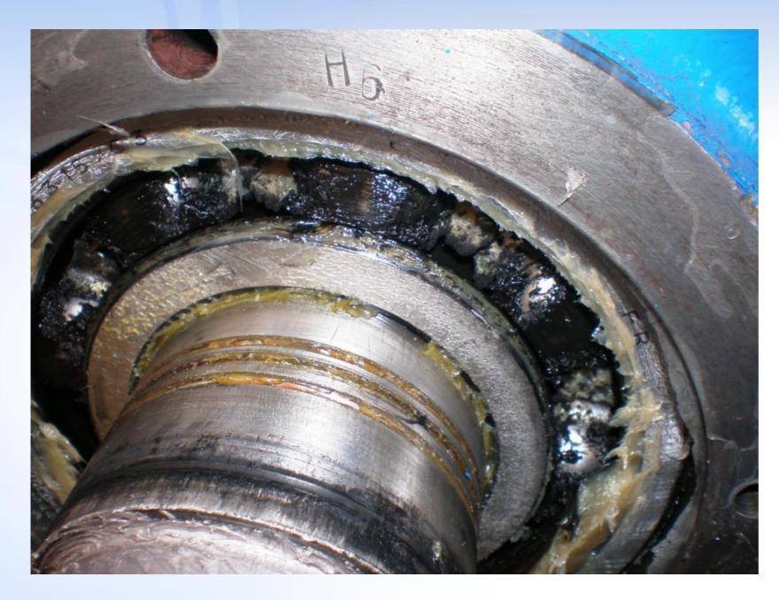
Typical example of burnt grease caused by current discharge (drive of an extruder)
