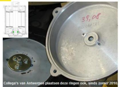
AEGIS® SGR-11.2-2 ring mounted in the end cap of the gear box in 2009. Measurements in 2014 proved the effectiveness of the solution - <1 V pp
