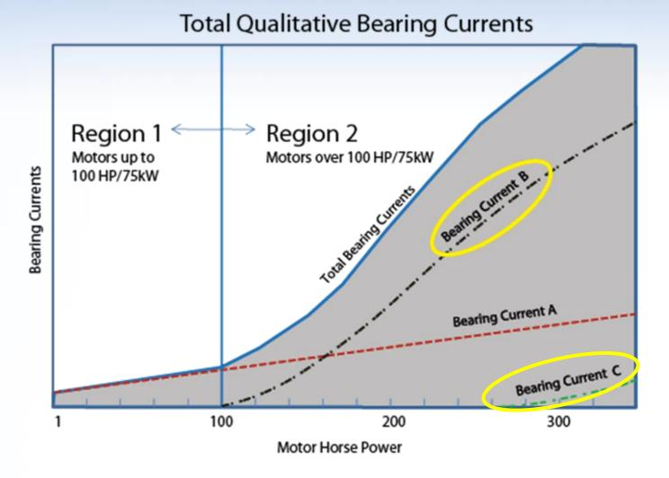
**Best Practice:** Interrupt the circuit by insulating one end (opposite to grounding side) – best with an insulated bearing.
