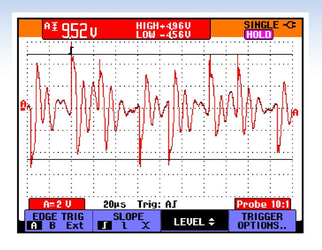
As discharges occur in the bearings, the lubrication is contaminated with carbon and metal particles. The lower impedance to the shaft voltages results in lower peak to peak voltages. This condition is usually found in motors that have been in operation for many months or years.
