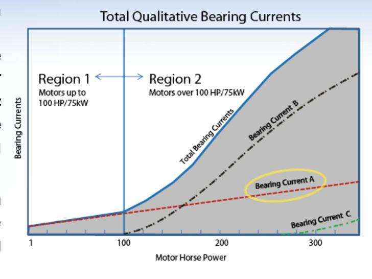
**Best Practice:** Ground the motor shaft – best with the AEGIS® Shaft Grounding Ring to provide a path of least resistance to ground and divert current away from the motor's bearings and to protect attached equipment. (Ref: NEMA MG1 Part 31.4.4.3)
