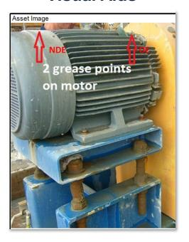
With a very simple work instruction, the maintenance tech is equipped with the information necessary to carry out a precision lubrication – no guesswork!
