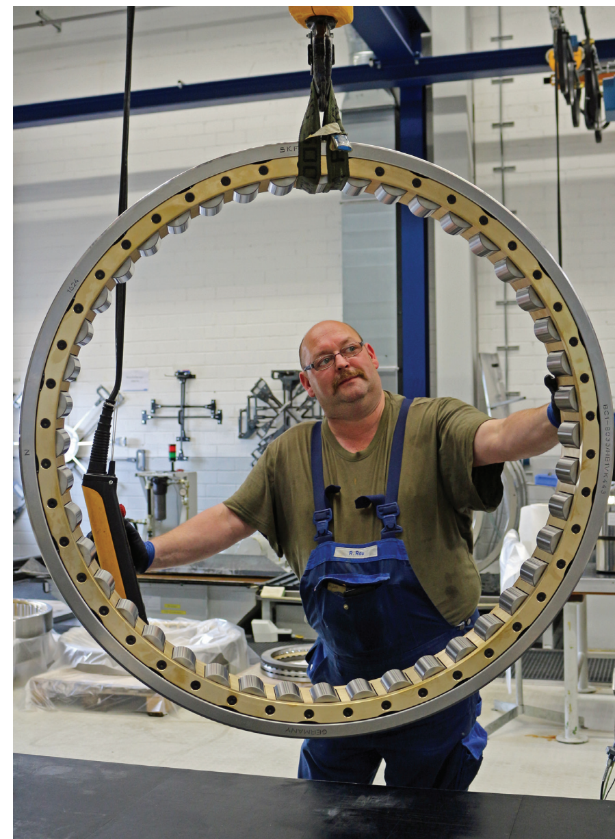
The new LSB test centre completes the engineering and production capabilities that SKF has concentrated at its Schweinfurt site. The findings from the new test centre will also be used to optimise the large self-aligning roller bearings (right picture) produced in Göteborg, Sweden.
